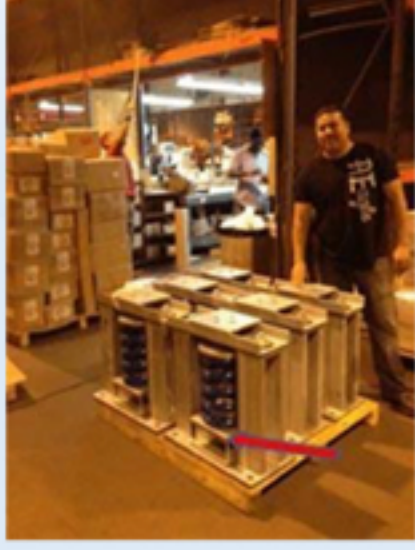
Chain hoists were required to maneuver these monsters into position for welding. Completed isolators weighed more than 400 lbs. each.
