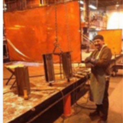
Chain hoists were required to maneuver these monsters into position for welding. Completed isolators weighed more than 400 lbs. each.
